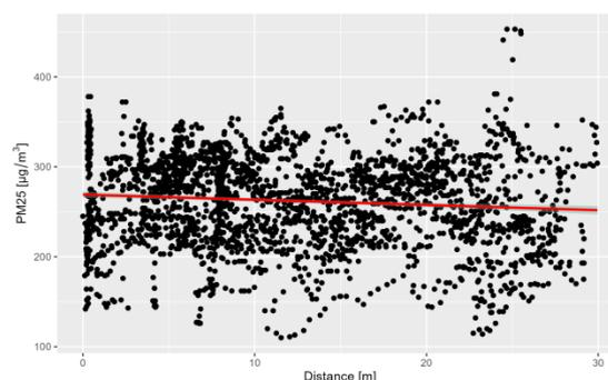
Fig. 7.  $\text{PM}_{2.5}$  concentration with increasing distance from the road – cool period
