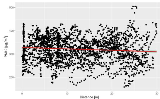
Fig. 8. PM<sub>10</sub> – concentration with increasing distance from the road – cool period
