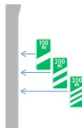
Fig. 2. Experimental marking: Pre-signpost board on the expressway (E-1 sign, on the left) and countdown markers (on the right)
