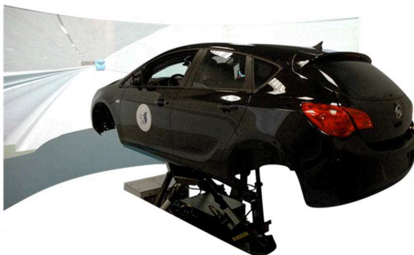
Fig. 1. AS1200-6 passenger car simulator. Source: Motor Transport Institute
