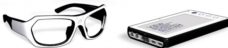
Fig. 3. Viewpoint System VPS 16 eye tracking device: glasses and smart unit
