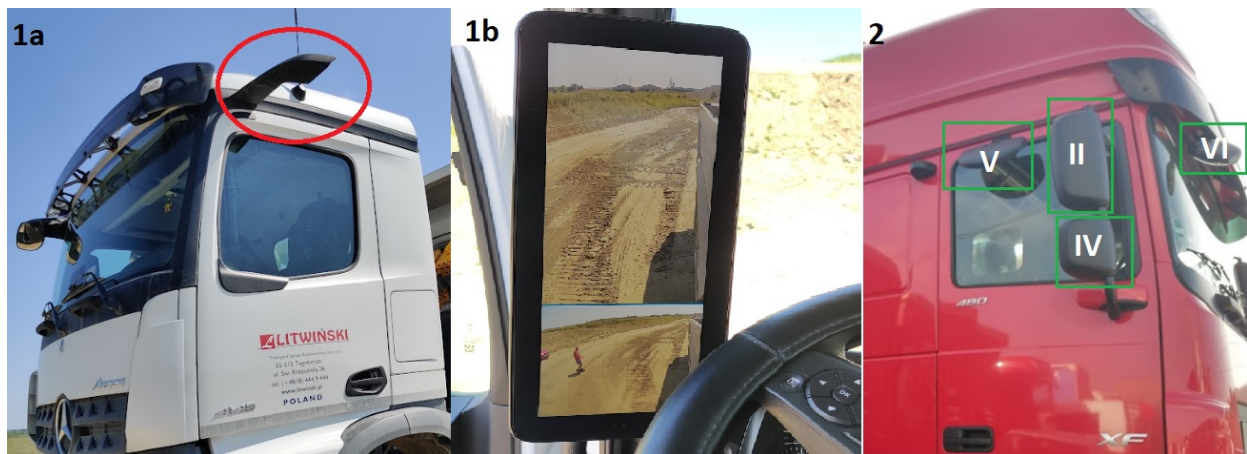
Fig. 4. The placements of the camera (1a) and screen (1b) in the camera-monitor system, as well as the placements of exterior mirrors and (2): II – Class II main mirror; IV – Class IV wide-angle mirror; V – Class V close-proximity mirror; VI – Class VI front mirror
