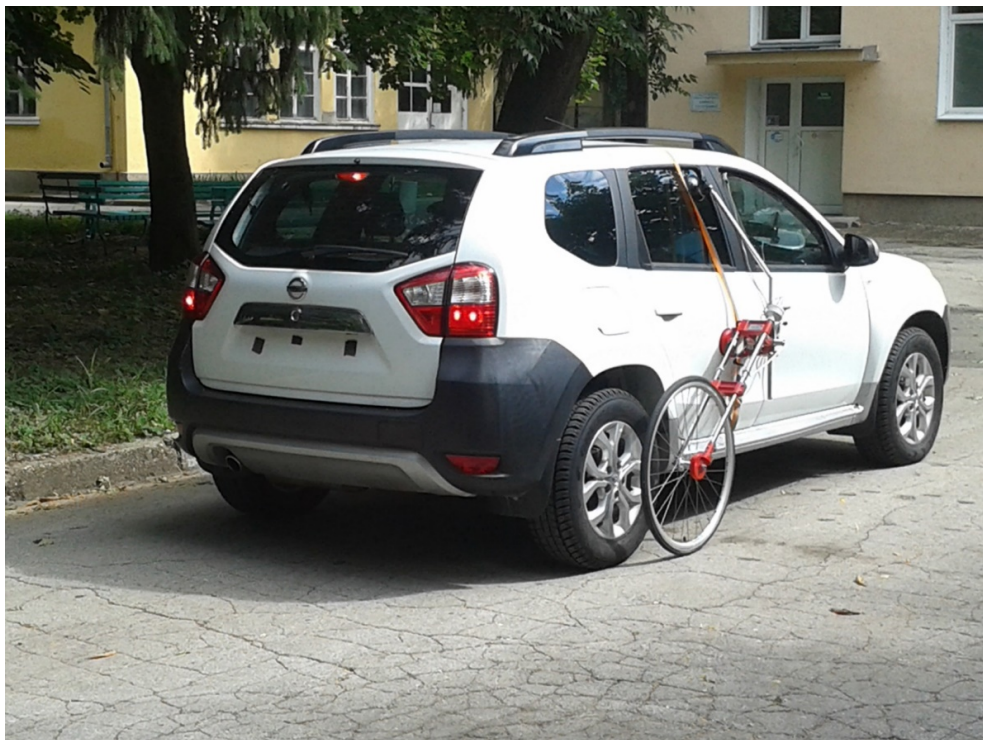
Fig. 5. Testing system with a “fifth” wheel mounted on the car with ABS
