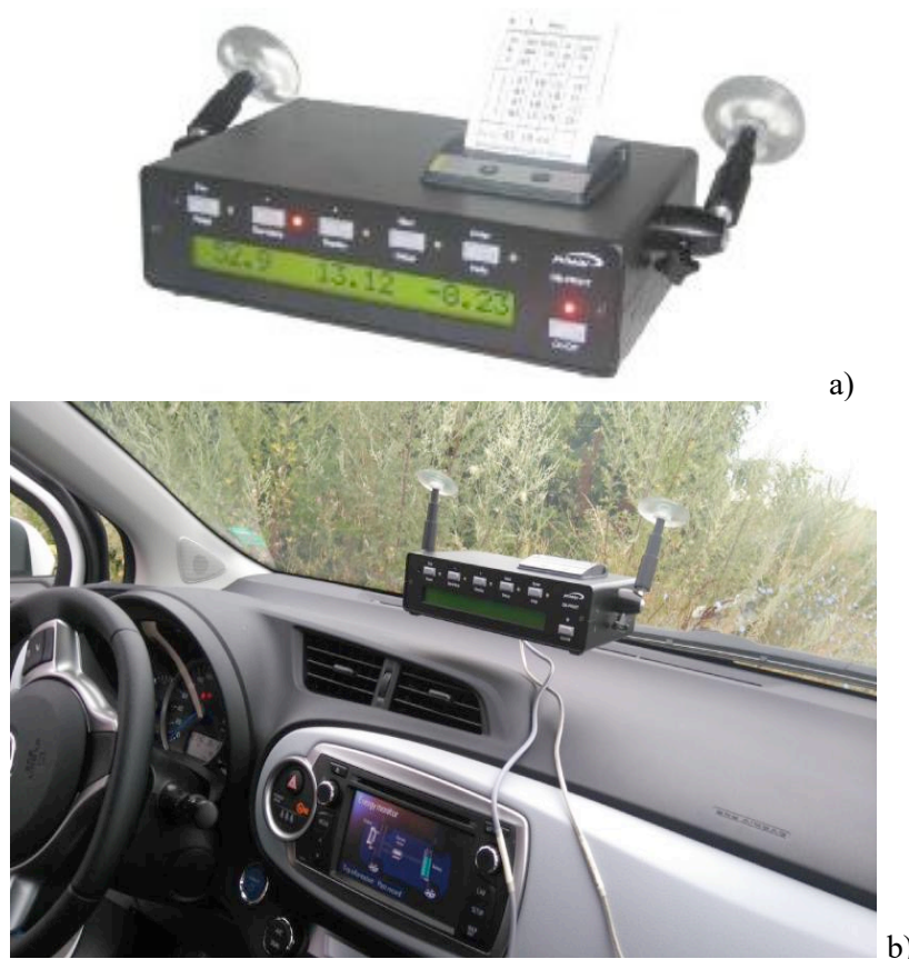
Fig. 6. (a) General view and (b) placement of DB Print device in the car during tests
