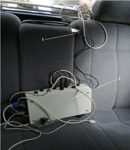
Fig. 3. Placement of (1) the piezo sensors and (2) the adapter in the car
