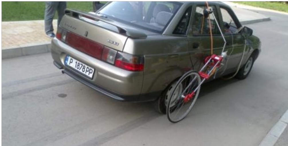
Fig. 4. Testing system with a “fifth” wheel mounted on the car without ABS
