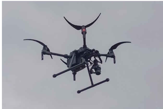
Fig. 1. DJI Matrice 210 v2 unmanned aerial vehicle during photogrammetric flight
