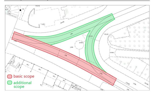
Fig. 1. The scope of the task "Replacement of turnouts in the junction of the Zwierzyniecki Bridge Mickiewicza Street with a task covered by the option right"
