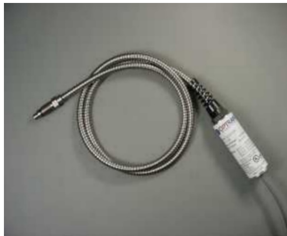
Fig. 4. Dynamic pressure sensor AutoPSI-S by "Optrand"
