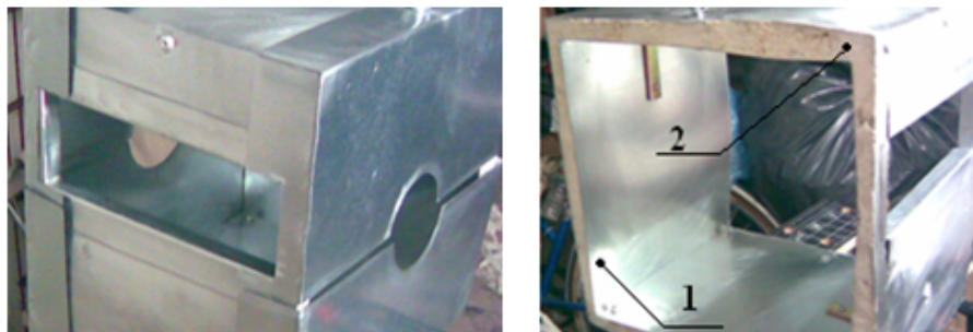
Fig. 5. Thermal chamber for a torsionally flexible coupling: 1 - sheet metal, 2 - polyurethane foam
