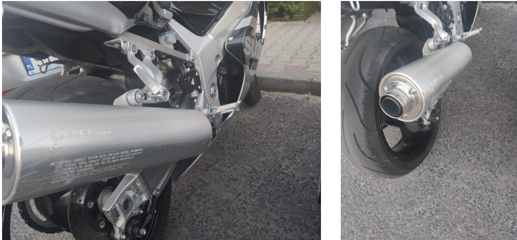
Fig. 3. A motor vehicle end muffler tip made of stainless steel
