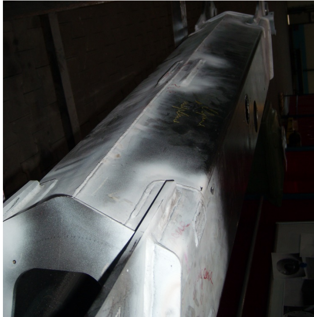
Fig. 1. Visible corrosion in the central part of the mobile platform (specific means of transport)
