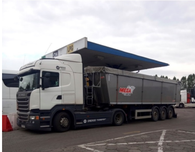
Fig. 10. A vehicle with highly loaded elements of a tipper made of austenitic steel
