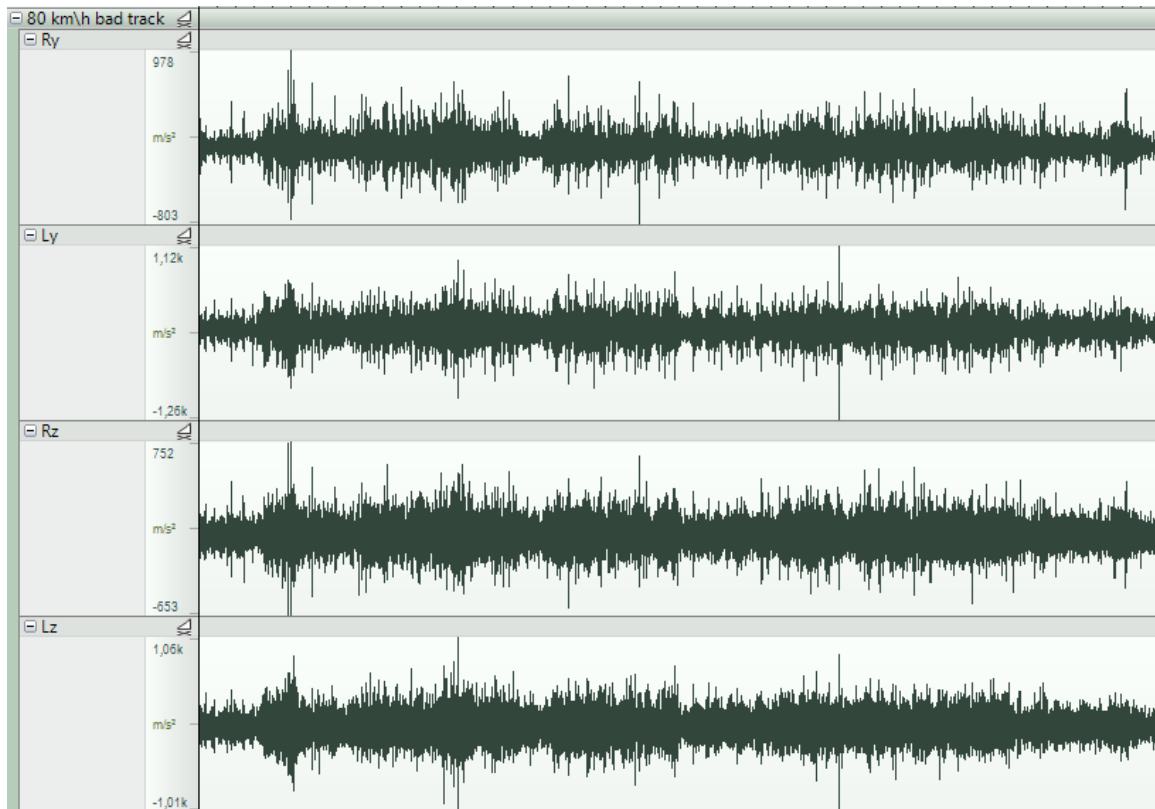
Fig. 4. Example of the recorded raw vibration signals [ \text{m/s}^2 ]
