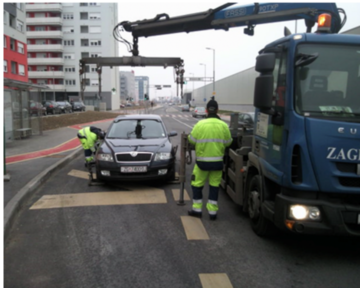
Fig. 2. Sideways vehicle loading using hydraulic stabilisers
