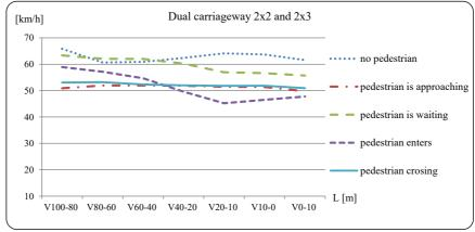
Fig. 9. Vehicle speed characteristics in the area of pedestrian crossings - permitted speed 50 km/h –average speed [12]
