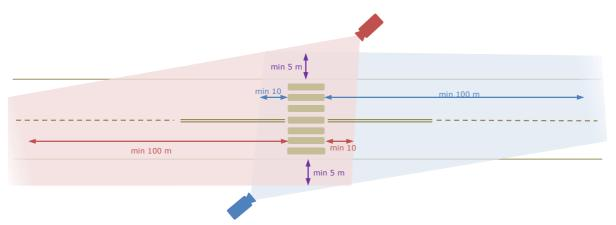
Fig. 5. Camera installation method - top view [12]
