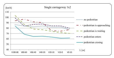
Fig. 10. Characteristics of vehicle speed in the area of pedestrian crossings - permitted speed 70 km/h - average speed at a distance up to 100 m before and up to 10 m after the pedestrian crossing [12]
