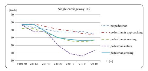
Fig. 11. Vehicle speed characteristics in the area of pedestrian crossings - permitted speed 50 km/ h - average speed at 100 m before and up to 10 m after the pedestrian crossing [12]
