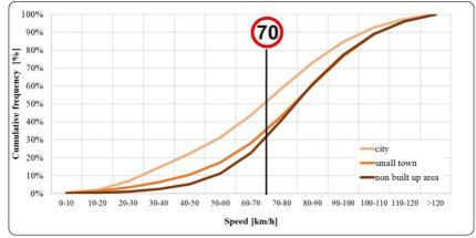
Fig. 8. Distribution of a speed of 10 m before pedestrian crossings in built-up areas and small towns - Vlimit = 70 km/h [12]
