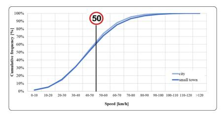
Fig. 7. Distribution of a speed of 10 m before a pedestrian crossing in cities and small towns – V limit = 50 km/h [12]
