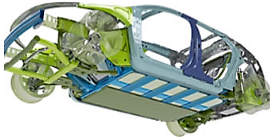
Fig. 1. Newest generation of steel in a car body structure [13]
