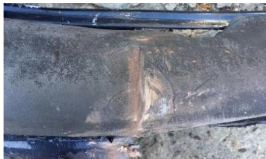
Fig. 3. Vehicle bumper paint layering due to an impact into a fencing pillar
