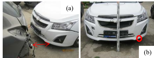
Fig. 10. Characteristic damage to Chevrolet and Opel vehicles
