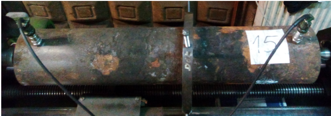
Fig. 7. Roller number 15 with visible transducers mounted above the bearing nodes during the measurement of vibration accelerations
