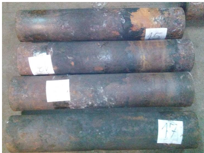
Fig. 4. Examined rollers with clearly visible marks of wear of jacket surface
