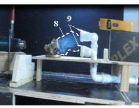
Fig. 2. Formation of the polluted zone: a – the exhaust fan does not work; b – the exhaust fan operates without guide plates t=14 s; c – the exhaust fan operates with the same guide plates t=14 s [21-22]
