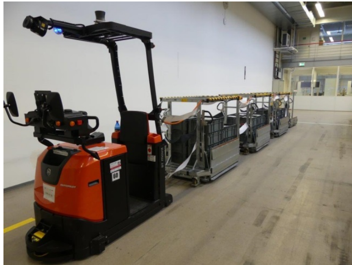
Fig. 1. Depiction of the type model of an autonomous logistics train set. Source: Authors, according to [1]
