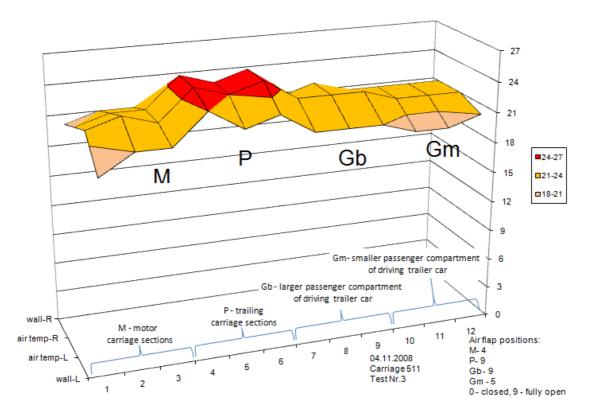
Fig. 2. Distribution of passenger compartment mean interior temperatures along the three carriages consist, train DR1B-511, test Nr.3 carried out on 04.11.2008 with outside air temp. of +2°C
