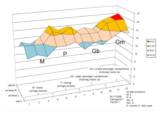
Fig. 1. Distribution of passenger compartment mean interior temperatures along the three carriages consist, train DR1B-511, test Nr.1 carried out on 04.11.2008 with outside air temp. of +2°C
