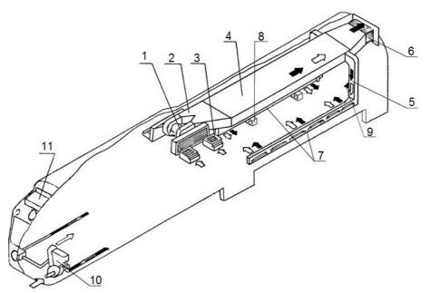
Fig. 3. Overall view of heating system of DR1AC train motor carriage, reproduced from [8]. 1 – centrifugal air blower, 2 – connecting air ducts, 3 – fresh air filters, 4 – main air duct, 5 – vertical branch air ducts, 6 – flexible air ducts for coupling between carriages, 7 – horizontal air ducts for distribution of hot air, 8 – electric blowers, 9 – air flaps, 10 – cabin heater, 11 – cabin air conditioner
