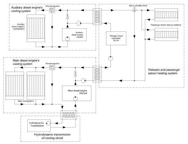
Fig. 4. Simplified hydraulic scheme of main and auxiliary diesel engine cooling systems and Webasto & passenger saloon heating system of the DR1AC series modernized DMU train.
