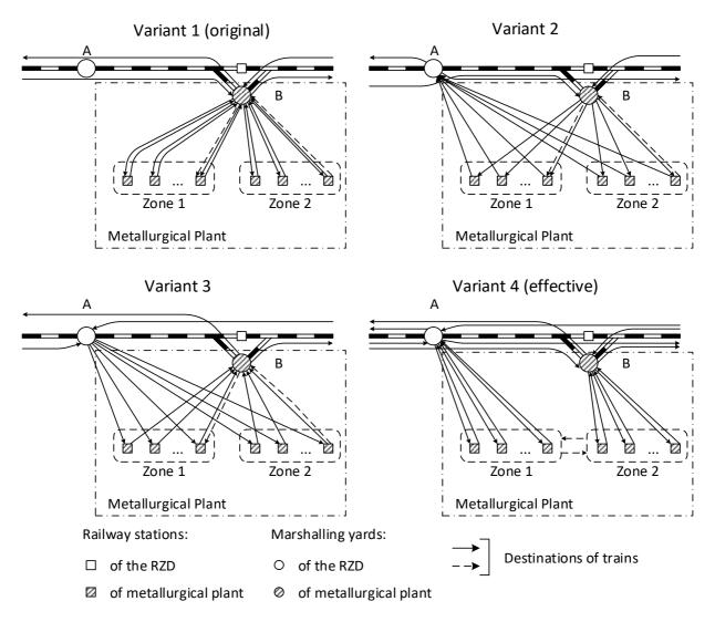
Fig. 1. Variants of distribution of marshalling work
