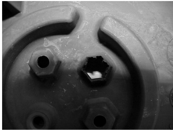
Fig. 2. Element damage occurred after anodizing in other acids than H_2SO_4
