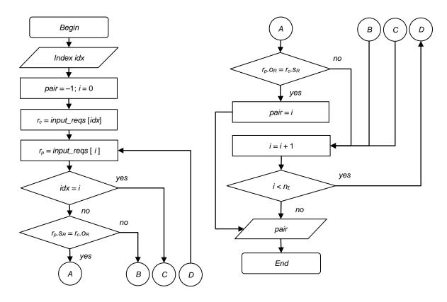
Fig. 2. Algorithm of the pair(\$idx) function
