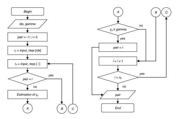
Fig. 3. Algorithm of the *circ\_pair*(\$idx,\$gamma) function
