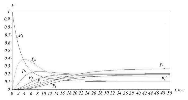
Fig. 7. The dependency of probabilities of the rail module states without running gear change in operation on service time
