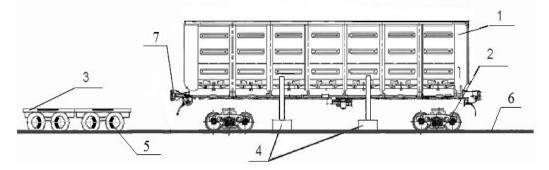
Fig. 1. Change from rail running gear to truck running gear on the extended jacks: 1 – open wagon; 2 – rail running gear; 3 – truck running gear; 4 – jacks; 5 – air brakes; 6 – railhead level; 7 – rotating automatic coupling device of the wagon
