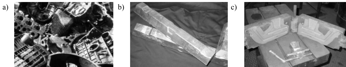
Fig. 3. Production of experimental material A226 cast alloy: a) aluminium scrap; b) ingot of experimental material; c) permanent mould and cast of A226
