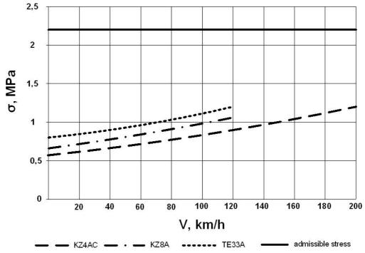
Fig. 3. Stress under rail bearing plates
