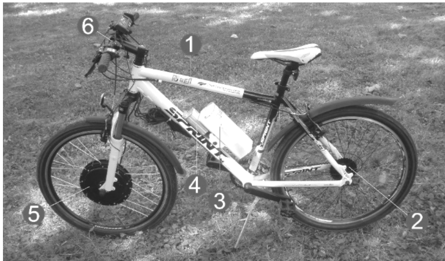
Fig. 1. General view of the electric bicycle: 1 – frame; 2 – back wheel with a chain mechanism; 3 – battery; 4 – controller; 5 – electric motor; 6 – handlebar
