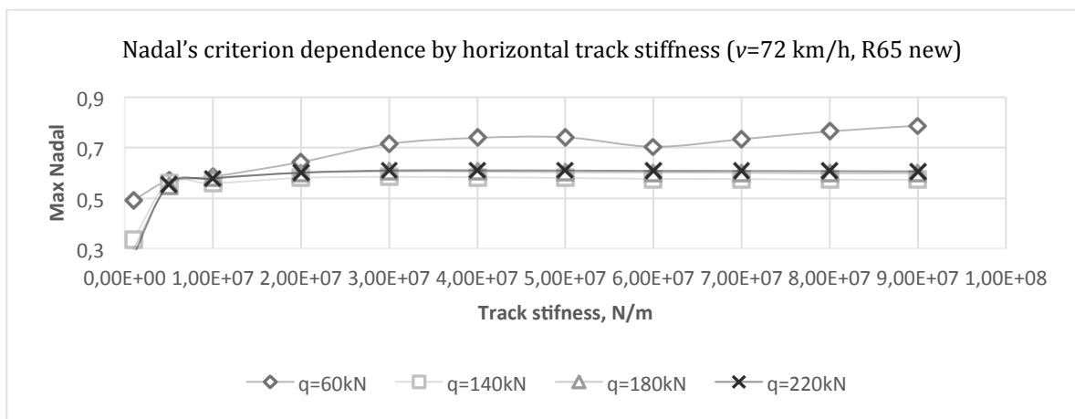
Fig. 16. Nadal's criterion dependence by track horizontal stiffness in curve ( v=72 km/h, R65 new)
