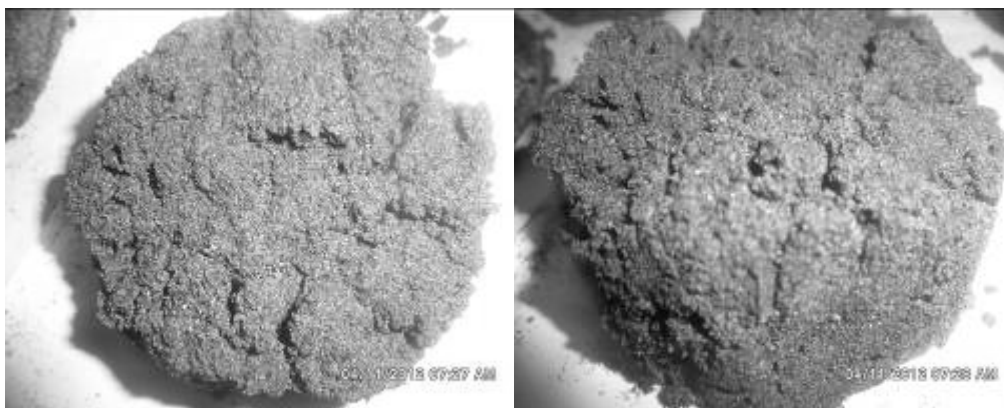
Fig. 5. View of the protective layer on the border line of impregnation in the wet sand: a) top view; b) side view
