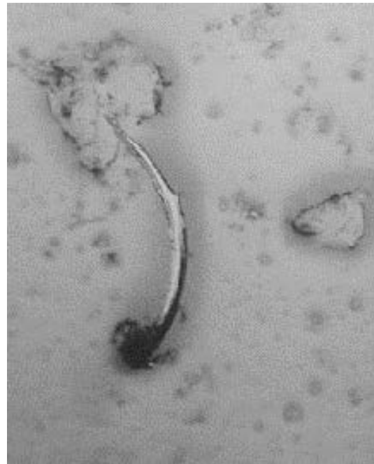
Fig. 4. Strong cutting wear steel particle, so-called two-point abrasion. Harder member of the friction pair penetrates into softer member of friction pair and separates chips from it. Magnified 1000x
