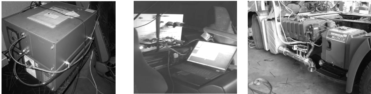
Fig. 4. Mobile measuring device, equipment in a vehicle cabin and on exhaust system (from left to right)
