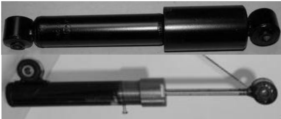
Fig.1. The rear shock absorber before and after modification
