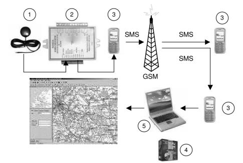
Fig. 3. Measuring path for appointing the distance with the geographical coordinate use: 1 – GPS aerial, 2 – GPS module, 3 – GSM phone, 4 – specialist software, 5 – PC class computer
