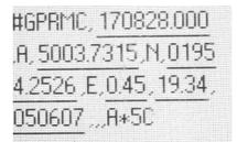
Fig. 6. The SMS screen with the information about the location with the use of the NMEA standard (for the point of measuring no II - Fig. 5)
