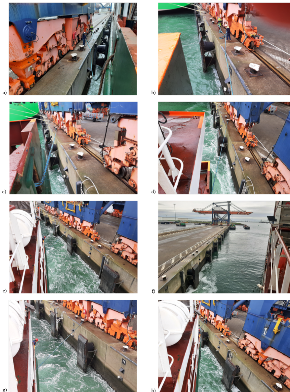
Fig. 6. Procedure of unberthing using the aft spring: (a) sending the aft spring to the quay in the position of the stern line; (b) the aft spring sent to the quay in the position of the stern line; (c) taking in the slack on the mooring line; (d) moving the bow away from the quay; (e) moving the bow to the largest possible angle away from the quay – the view from the stern; (f) moving the bow to the largest possible angle away from the quay – the view towards the bow; (g) moving the bow away from the quay to the maximum angle of
