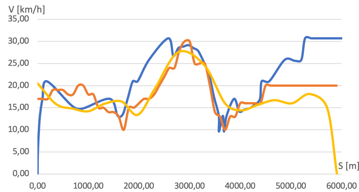
Fig. 5. Diagram of the dependence of the TEM2 locomotive start-up on the resistance to motion arising during the start-up of the locomotive with a given load
