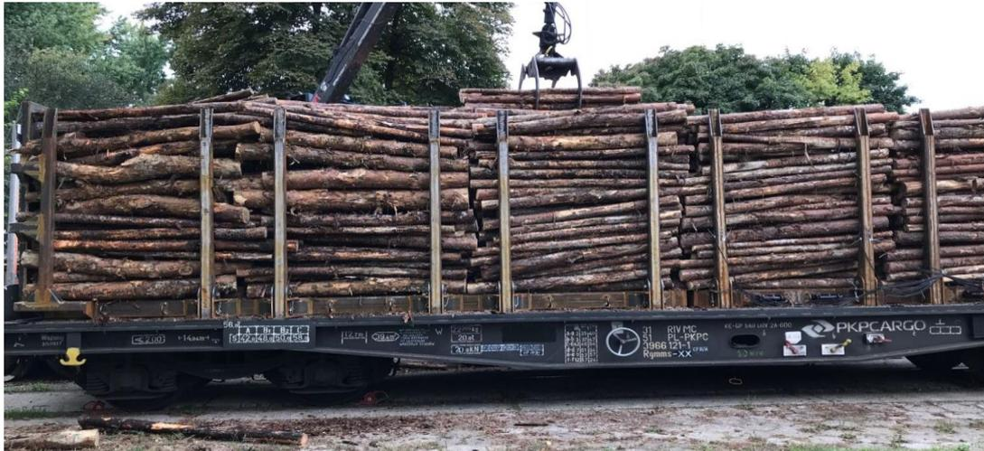
Fig. 12. Loading of timber into stanchion baskets on a platform wagon
