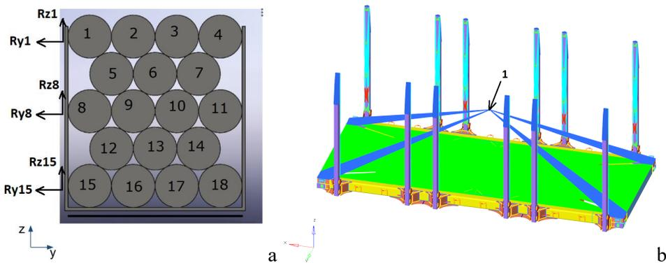
Fig. 6. Bin load models: a) log load and b) container load
