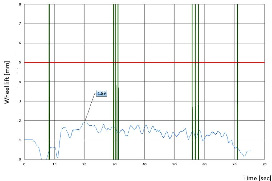
Fig. 9. Lifting of the platform guide wheel during passage 3 through an arc with radius  $R = 150$  m
