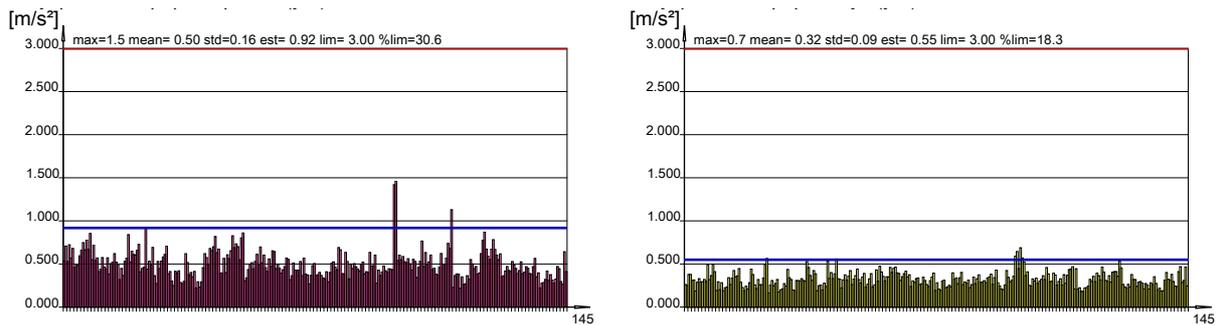
Fig. 14. Transverse acceleration waveforms recorded on the body of a wagon with a basket installed on
