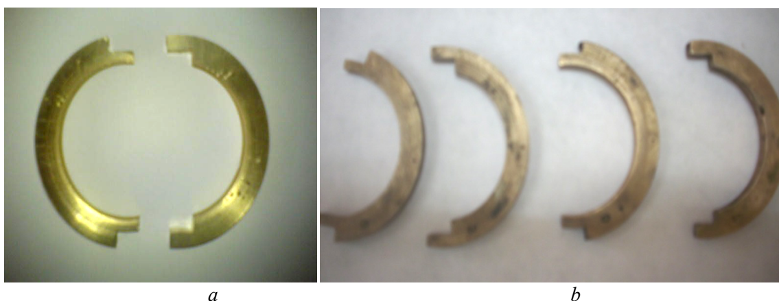
Fig. 2. Half-rings for sealing the piston in the cylinder: a) two half-rings for creating a ring of the same level b) a complete set of half-rings for sealing one piston
