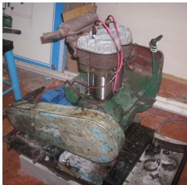
Fig. 5. The reconstructed engine used to study the dry sealing of the piston in the cylinder
