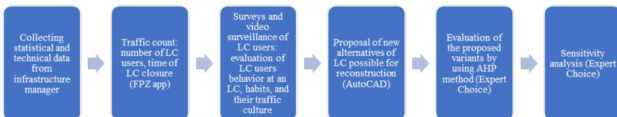
Fig. 1. Case study: steps for the evaluation of a level crossing design
