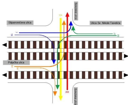
Fig. 3. Load of traffic flows by motor vehicles in the morning peak hour
