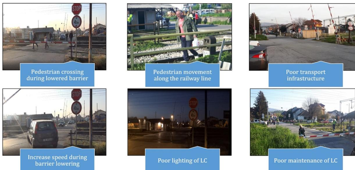
Fig. 2. Problems at LC Sokolska (poor infrastructure and level crossing users' behaviours)
