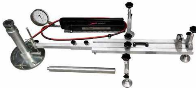
Fig. 4. Static plate load test device [28]
