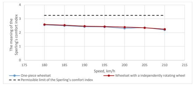
Fig. 11. Sperling's comfort index values in the vertical direction in the straight section
