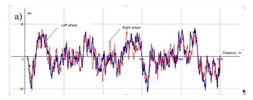
Fig. 5a. Vertical irregularities of the modeled track
