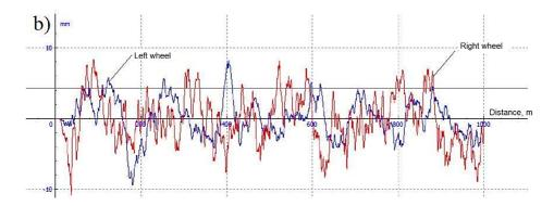
Fig. 5b. Horizontal irregularities of the modeled track
