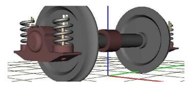
Fig. 2. Wheelset with independently rotating wheels
