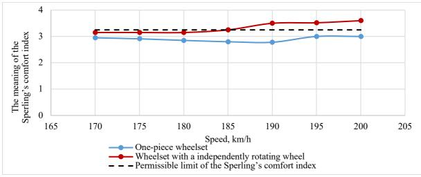
Fig. 10. Sperling's comfort index values in the lateral direction in the 2900 m radius curve
