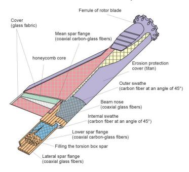
Fig. 9. Rotor blade of a modern helicopter [16]
