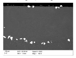
Fig. 13. The surface layer of AlSi9Cu alloy after melting the ceramic powder, laser power 1.5 kW, 1.5 g/min, remelting rate 0.25 m/min
