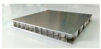
Fig. 2. A sample of radar absorbing honeycomb material [the authors own work]
