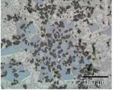
Fig. 4. Examples of Metal Matrix Composites a) ASCM alloy+SiC9%; b) AlSi25+SiC20% [the authors own work]
