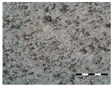
Fig. 3. Ceramic Matrix Composite F1200, with aluminium oxide matrix reinforced B<sub>4</sub>C [the authors own work]
