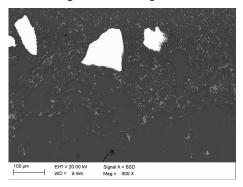
Fig. 14. The surface layer of AlSi9Cu alloy after melting the ceramic powder, laser power 1.5 kW, 1.5 g/min, remelting rate 0.25 m/min
