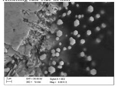
Fig. 16. Boundary of the powder-Al matrix of surface layer of AlSi9Cu alloy after melting the ceramic powder, laser power 2.0 kW, 8.0 g/min, remelting rate 0.25 m/min
