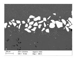
Fig. 12. The surface layer of AlSi9Cu alloy after melting the ceramic powder, laser power 2.0 kW, 1.5 g/min, remelting rate 0.25 m/min
