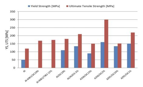
Fig. 5. Impact of the reinforcement type on the strength properties of composites; Al-6061/SiC12% reinforcement particle size 40-45  $\mu$ m; Al-6061 / TiB<sub>2</sub>-10% - 1-2  $\mu$ m; Al/SiC10% - 10  $\mu$ m; Al/Al<sub>2</sub>O<sub>3</sub> 2% - 25 nm; A356 / SiC15% - 40  $\mu$ m; A356/SiC2% - 20-30 nm; AZ91/SiC10% - 7 $\mu$ m; AZ91/SiC1% - 30 nm [12]
