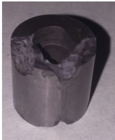
Fig. 1. Defective hard-alloy cutter rejected during operation of the mill to the KJ20 machine
