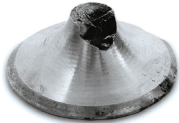
Fig. 1. Fatigue crack in the zone of transition of the cylindrical valve shaft into a valve head [15]
