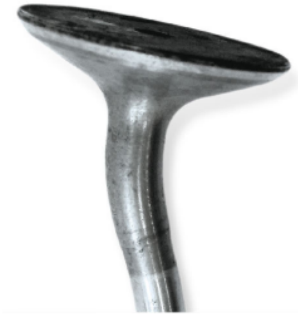
Fig. 2. Permanent bending of the valve shaft [15]
