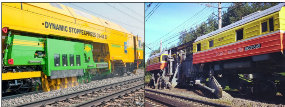
Fig. 2. Machines for continuous tamping (left – Dynamic Stopfexpress 09-4X [45], right – VPO-3000)
