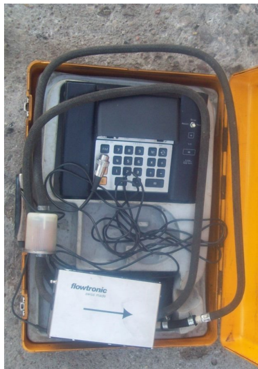
Fig. 2. Testing device for fuel consumption Flowtronic 205
