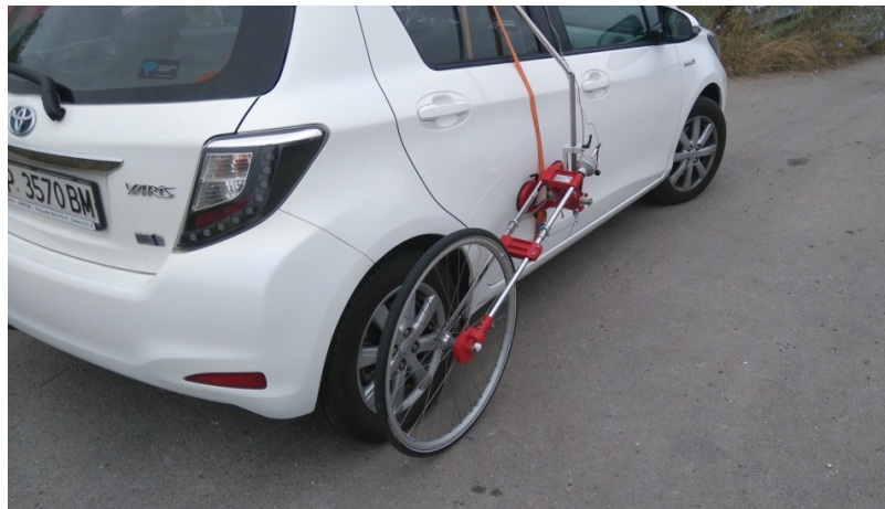
Fig. 1. Tested hybrid car Toyota Yaris Hybrid 1.5 HSD with a “fifth” wheel Peiseler and system DB Print (in the car)
