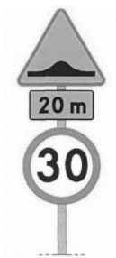
Fig. 3. Vertical marking of the serial release ramp, in which the distance between consecutive thresholds is not less than 20m and with a speed limit of 30km/h [12]
