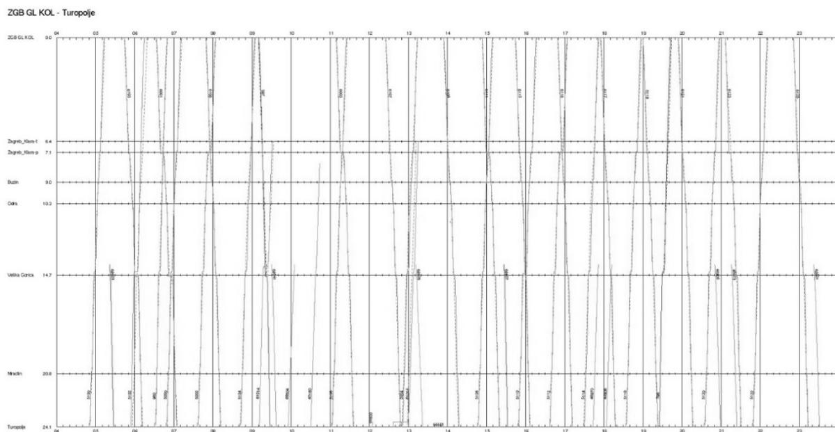
Fig. 2. Timetable graph for 2016/2017 for the line section Zagreb Glavni – Turopolje obtained by simulation in the OpenTrack program
