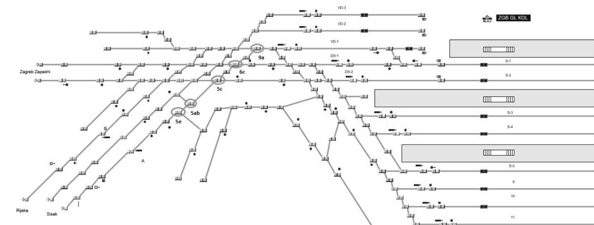
Fig. 3. Changes in the model of the current condition of the Zagreb Glavni railway station infrastructure
