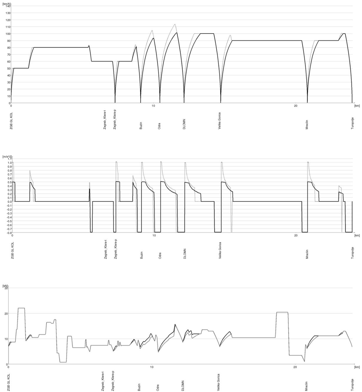
Fig. 8. Comparison of speed, acceleration and track resistance profiles for EMUs HŽ 6112 (grey line) and HŽ 6111 (black line)
