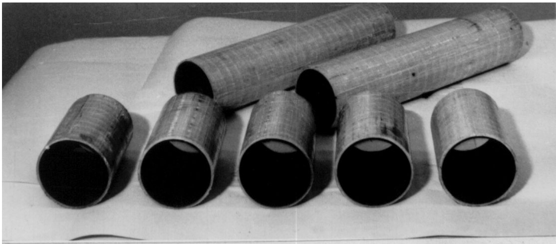
Fig. 5. Photo of metal-fiberglass pipe samples (fragments)
