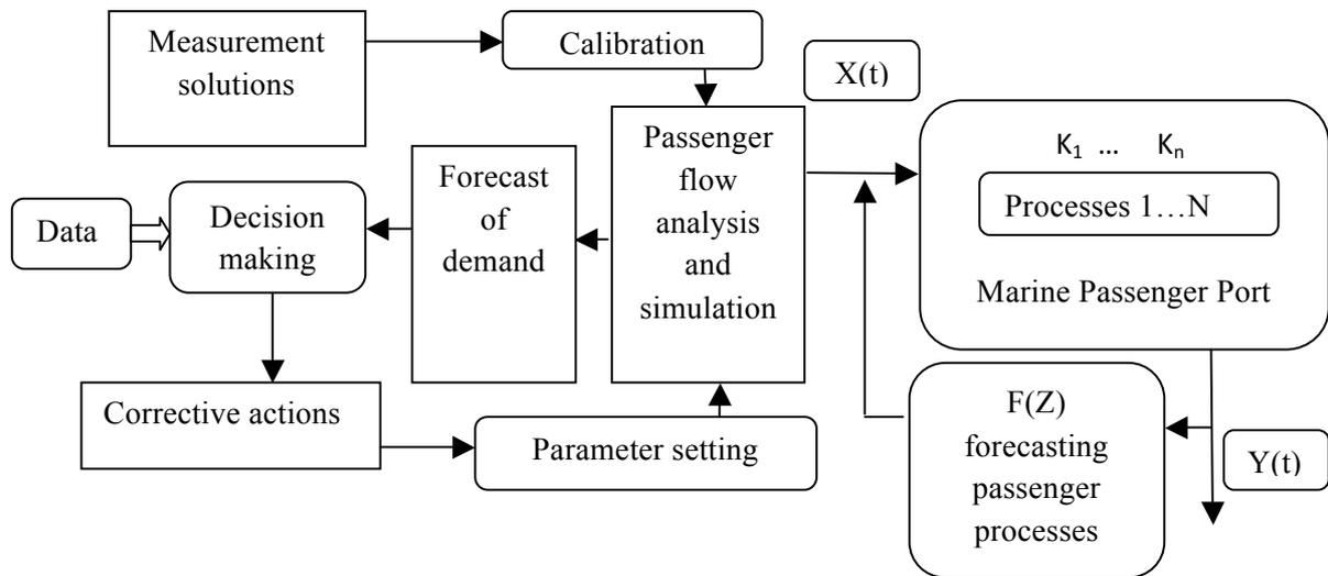
Fig. 2. Block for forecasting passenger processes in the terminal structure
