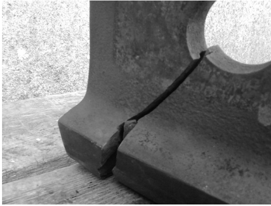
Fig. 5. The cut specimen of the wing under the defect code U.53.2
