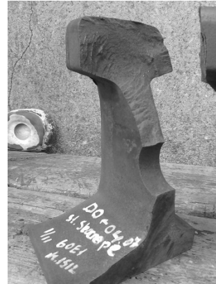
Fig. 6. The part of the cut broken wing (end view)
