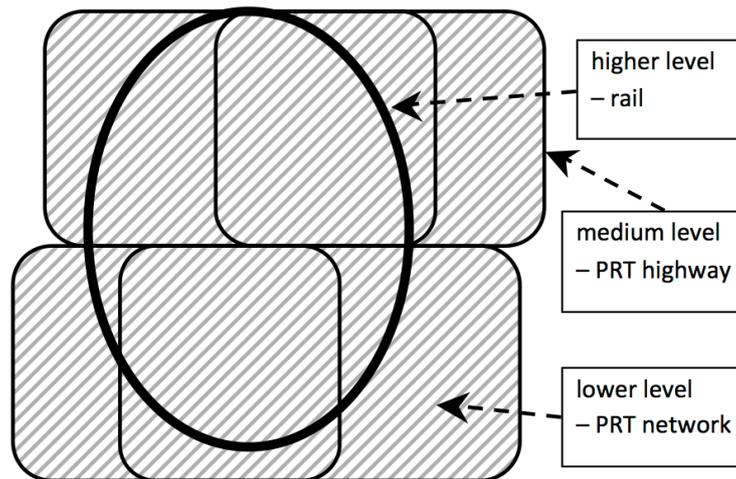
Fig. 1. A schematic of light rail ring (oval) and PRT commuter network (rounded boxes)
